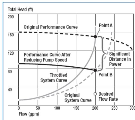
**Fig. 4.** Affinity laws and energy savings when use VSD compare with throttling control
