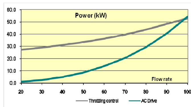
**Fig. 5.** Energy consumption with throttling control and VSD for different flow rate
